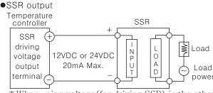
\*When using voltage (for driving SSR) in the other purposes, do not over the range of rated current.
